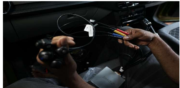
STEP 14 :- CONNECT THE 4 CAMERAS ( AS MARKED BY THE STICKERS) TO THE CAMERA CORD AS MARKED IN STEP 13
