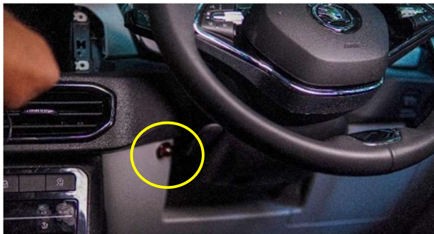
STEP 89 :- CLEAN THE AREA HIGHLIGHTED WITH THE ALCOHOL SWAB THAT IS PROVIDED AND WAIT FOR 1 MINUTE THEN, STICK THE REMOTE SENSOR, AS ABOVE LOCATION AS SHOWN.
