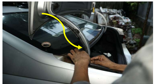
STEP 66 :- ROUTE CABLE AS SHOWN FROM HOLES IN TAIL GATE.
