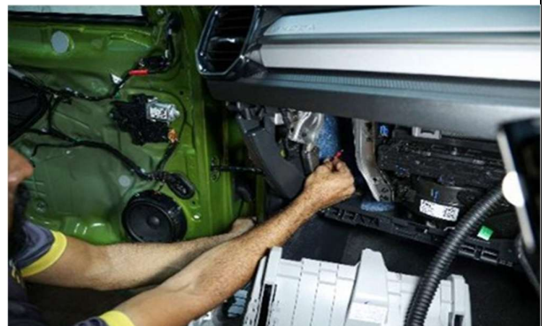
STEP 51 :- AFTER ROUTING THROUGH THE HOLE, PULL ALL THE EXCESS CABLE GENTLY
