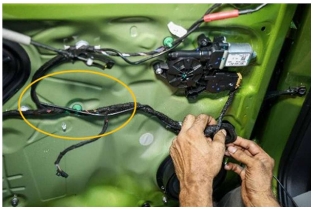
STEP 46 :- ROUTE THE EXTENSION CABLE WITH THE SERIES CABLE.
