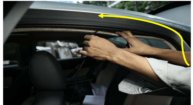
STEP 70 :- ROUTING CABLE THROUGH THE ROOF LINER FROM REAR DOOR TO FRONT DOOR.
