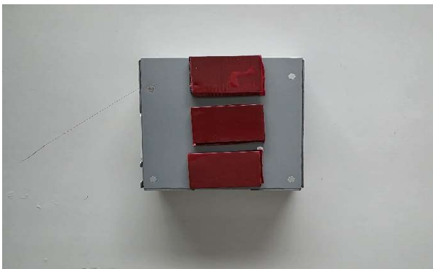
STEP 101 :- STICK THE DSA TAPE (PART NUMBER 14) ON THE JUNCTION BOX AS SHOWN
