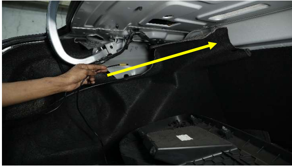
STEP 67 :- ROUTE EXTENTION CABLE YELLOW (PART 4) MALE END THROUGH THE RUBBER SLEEVE
