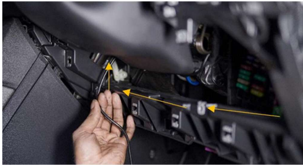
STEP 56 :- ROUTE CABLE AS SHOWN UNDERNEATH STEERING COLLUMN.
