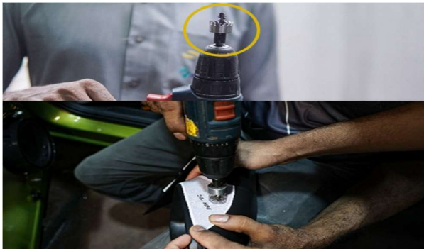
STEP 34 :- DRILL THE HOLE USING HOLE SAW 22.5 MM (PART 13) AS PER MARKINGS GIVEN ON THE TEMPLATE.
