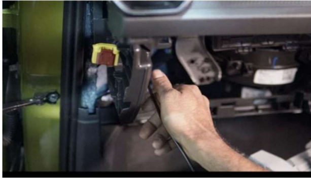
STEP 85 :- PASS THE CABLE THROUGH RUBBER SEAL AND THE GLOVEBOX ARE (KINDLY REFER TO THE VIDEO IF ANY CONFUSION.
