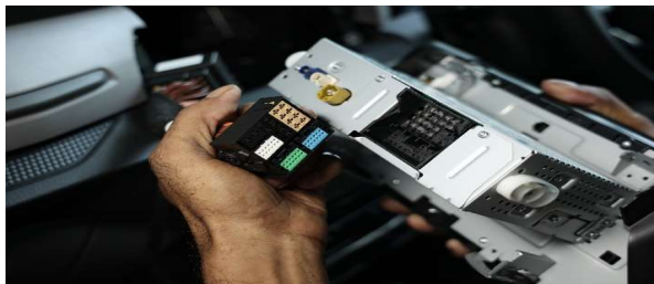
STEP 7 :- CONNECT THE OTHER END OF ( PART 9 ) TO THE SERIES MULTIMEDIA/INFOTAINMENT AS SHOWN ON THE STICKER.
