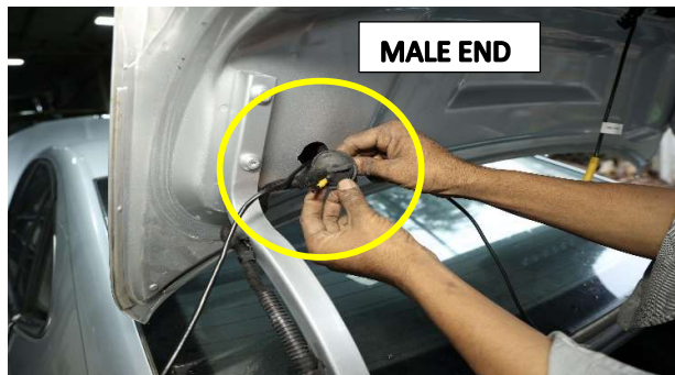
STEP 65 :- ROUTE EXTENSION CABLE YELLOW (PART 4) MALE END AS SHOWN FROM HOLES IN TAIL GATE.
