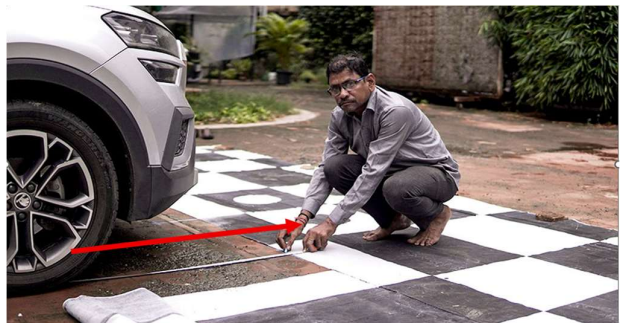
STEP 106 :- MEASURE FROM THE TYRE 35 INCHES AND ALIGN THE MAT 35 INCHES FROM THE BOTH FRONT TYRES. MAT HAS TO BE PLACED. (PLEASE REFER TO THE VIDEO FOR REFERENCE).
