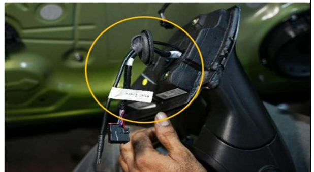
STEP 39 :- ROUTE CABLES AS SHOWN FROM RUBBER GROMMET
