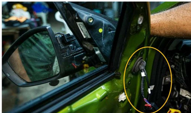
STEP 40 :- CONNECT THE LEFT AND RIGHT ORVM's AND ROUTE CABLES AS SHOWN.
