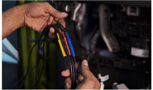
STEP 86 :- CONNECT ALL 4 CAMERA EXTENTION CABLES (PART 2,3,4,5 )TO THE 32 PIN CONTROL CORD (PART 6) AS SHOWN.
