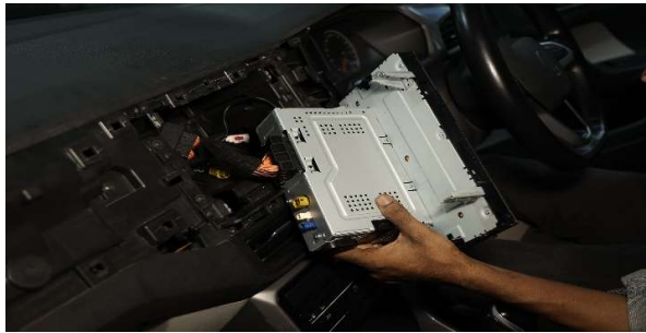
STEP 5 :- DISCONNECT ALL SERIES CABLE FROM MULTIMEDIA/INFOTAINMENT
