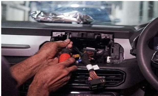
STEP 103 :- FITMENT OF MULTIMEDIA/INFOTAINMENT AS PER SERIES PROCESS
