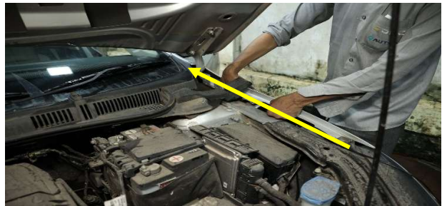
STEP 82 :- ROUTE FRONT EXTENSION CABLE (PART 5) THROUGH EDGES OF THE ENGINE BAY
