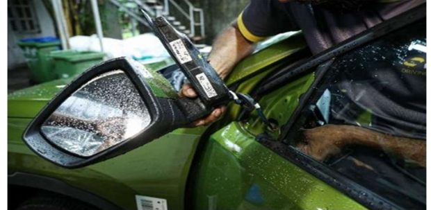
STEP 31:- REMOVE THE LEFT AND RIGHT ORVM's CAREFULLY AS PER SERIES PROCESS.
