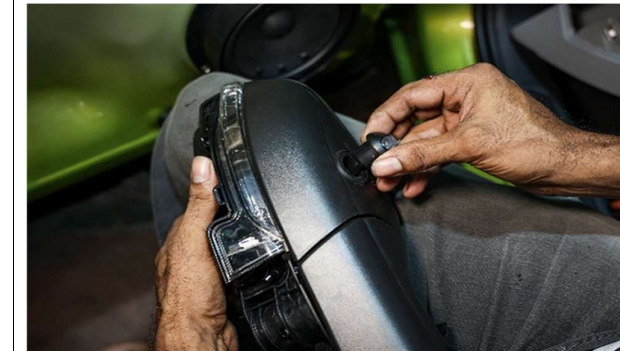
STEP 35 :- INSERT LEFT AND RIGHT CAMERA IN ORVMs RESPECTIVELY WITH RUBBER COVER/CAP ON THE CAMERA.
