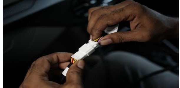
STEP 10 :- CONNECT THE 2 SOCKETS AS MENTIONED ON THE PARTS STICKER
