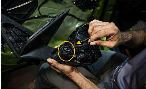
STEP 36 :- ROUTE THE CABLES THROUGH SPACE MARKED ( FOR CLEAR DEMONSTRATION KINDLY REFER TO THE INSTALLATION VIDEO)
