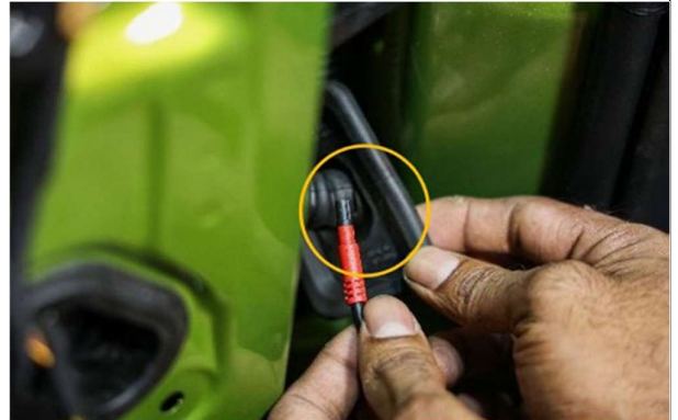
STEP 49 :- ROUTE CABLE THROUGH THE RUBBER PART AS SHOWN
