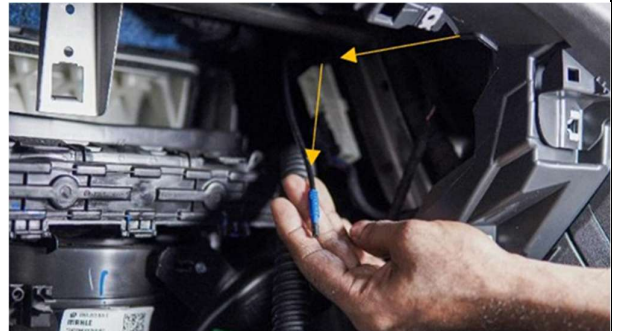
STEP 57 :- PASS THE CABLE TILL THE JUNCTION BOX AREA, JUST LIKE STEP 56
