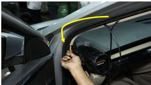
STEP 75 :- ROUTE CABLE UNDERNEATH THE A-PILLAR.
