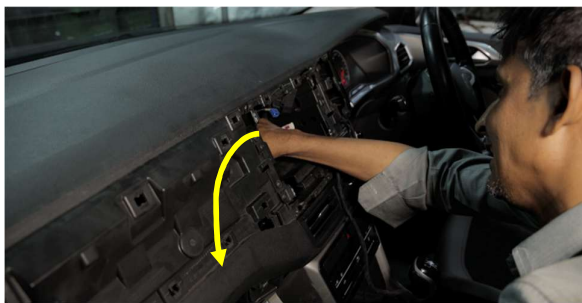
STEP 22 : - ROUTE SAVV DEDICATED POWER CABLE (PART 9 ) FROM THE BACK OF THE MULTIMEDIA/INFOTAINMENT TO THE GLOVE BOX AREA AS SHOWN
