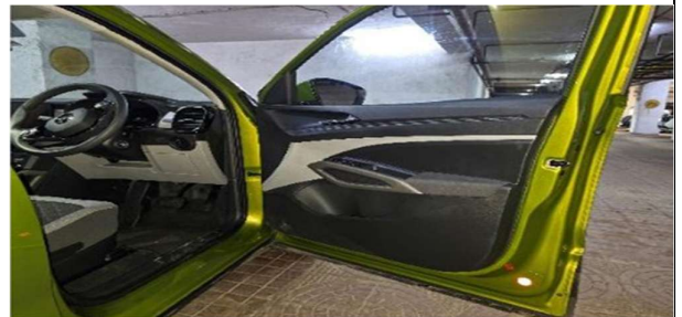
STEP 59 :- ASSEMBLE DOOR TRIM OF THE LEFT AND RIGHT DOOR + OVRM AS PER SERIES PROCESS AFTER ENSURING ALL ELECTRICAL CONNECTIONS.
